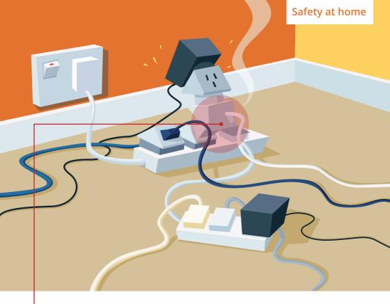
Never overload an extension lead by plugging in appliances that together will exceed the maximum current rating stated for the extension lead. This could make the plug in the wall socket overheat and possibly cause a fire. Use Electrical Safety First's socket calculator to check if you're exceeding the maximum load: www.electricalsafetyfirst.org.uk/ overloadingsockets
